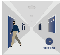
The sensor turns OFF light automatically after the holdtime when there's no motion detected.
